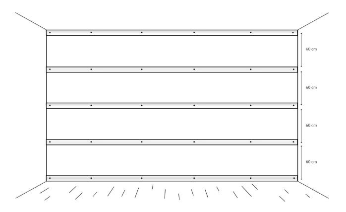
The first thing you need to do is to mount battens on the wall. This enables you to drill the screws through the felt of the **AkuTiles** and into the battens. Depending on the wall you will need plugs and and screws that fits accordingly to your wall type. We recommend that you keep a distance of 60 cm. between the battens.
