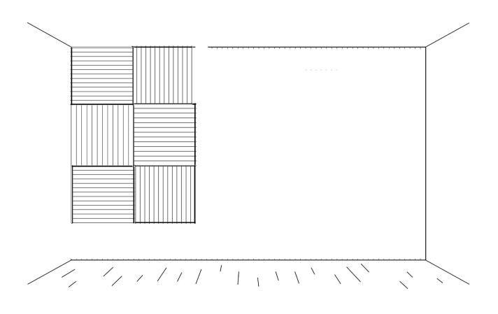
Mount the **AkuTile** on the wall by drilling the black screws (35 mm.) through the black felt and into the battens.
