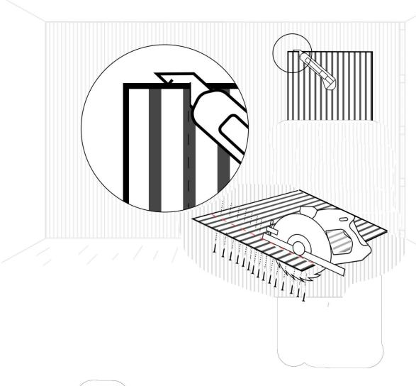
Adjusting the AkuTile sideways is done by cutting the panel in the felt using a knife or a saw.
