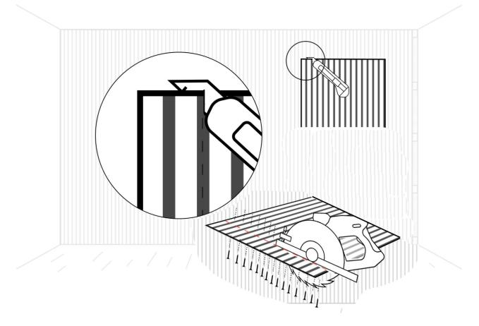
Adjusting the AkuTile sideways is done by cutting the panel in the felt using a knife or a saw.
