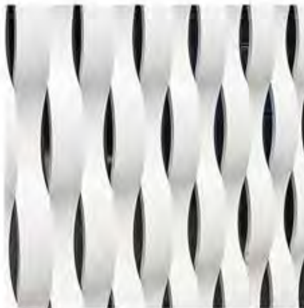
WAVY Shown in white paint finish. Nominal Panel Size: 48" x 96" Pattern Depth: Thru cut Panel Thickness: 3" nominal. Pattern Type: Repeating (4' x 8') only. Pattern direction – Vertical Only.
