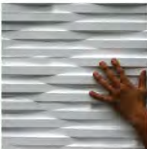
SST003 Shown in white paint finish. PD: Variable. PT: 0.75", 1", 1.5" Pattern Type: Repeating/Continuous. Pattern repeats every 96 inches parallel to direction of cut. Pattern bandwidth is 1 inch. Must be "A-B" panel match for horizontal repeat. Pattern direction may be selected in vertical direction or horizontal direction. Panel dimensions that are perpendicular to pattern direction need to be a multiple of two.
