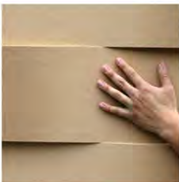
W1608 Shown unfinished HDF. PD: varies up to 1" depending on panel thickness. PT: 0.75", 1", 1.5". Pattern Type: Repeating 8" band on 16" wave. It is limited to 4'x8' or 4'x 10' panels only.
