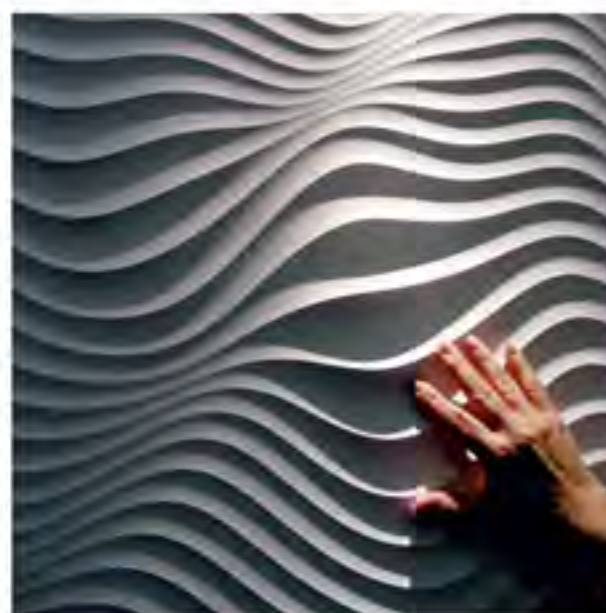
COU 001x2 Snow White membrane finish. PD: 1.2". PT: 1.5" Pattern Type: Continuous. Pattern is non-repeating. Panel layout must be submitted in order to achieve panel match. Pattern direction may be selected in vertical direction or horizontal direction.
