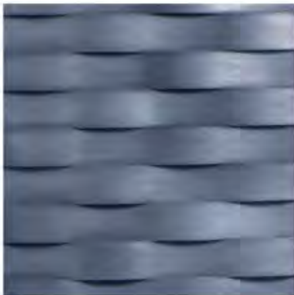
W1204 Shown in Barrel Steel Metallic paint. PD: varies up to 1" depending on panel thickness. PT: 0.75", 1", 1.5". Pattern Type: Repeating 4" band on 12" wave. It is limited to 4'x8' or 4'x 10' panels only.
