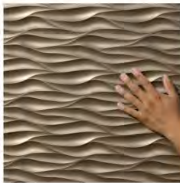
BIO 8 Shown in Bronze Metallic Paint. PD: 0.223". PT: 0.75". Pattern Type: Repeating. Pattern available in standard 48"x96" or 48"x120" panel sizes. Pattern repeats every 6 inches perpendicular to pattern direction and every 6 inches parallel to pattern direction. Pattern direction may be selected in vertical direction or horizontal direction.
