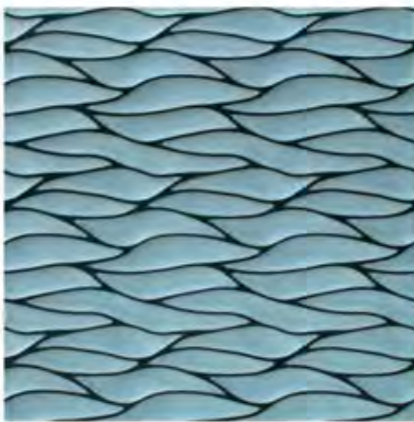
BIO 7 Clear/carved blue colored MDF PD: .4". PT: .75". Pattern type: repeating. Pattern available in standard 48"x96" or 48"x120" panel sizes. Pattern repeats every 12 inches perpendicular to pattern direction and every 12 inches parallel to pattern direction. Pattern direction may be selected in vertical direction or horizontal direction.
