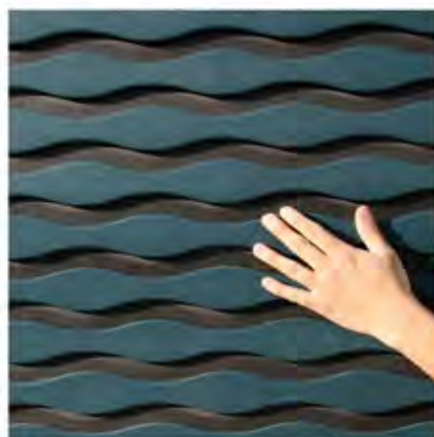
RBU305 Blue and black colored MDF / clear coat. PD: 0.5". PT: 0.75". Pattern Type: Repeating. It is limited to 4'x8' repeating panels only. Cannot be produced in different sizes.
