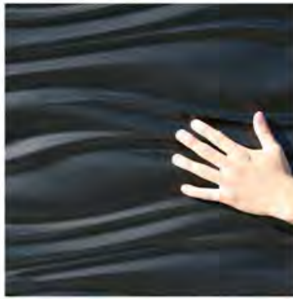
SOU017 Ebony Starlight membrane finish. PD: Variable. PT: 0.75", 1", 1.5" Pattern Type: Repeating/Continuous. Pattern repeats every 12 inches perpendicular to pattern direction and every 48 inches parallel to pattern direction.
